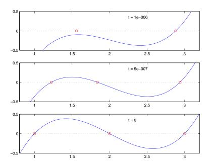
The bottom subplot shows the unperturbed polynomial, with its three roots at 1, 2, and 3. The middle subplot shows the first two roots approaching each other. In the top subplot, these two roots have become complex and only one real root remains.
