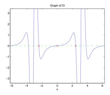
The red circles in the graph correspond to 2erosd(1), 2erosd(4), and 2erosd(5). As you can see in the graph, there are also 2eros at  $\pm\pi$ . The additional zeros occur because f'''(x) contains a factor of sin(x), which is zero at integer multiples of  $\pi$ . The function, solve(sin(x)), however, only finds the zero at x = 0.
