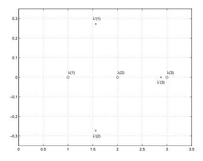
This, in turn, means that for some value of  $t = \tau$ ,  $0 < \tau < 10^{-6}$ , the perturbed matrix A(t) = A + tE has a double eigenvalue  $\lambda_1 = \lambda_2$ . The example shows how to find the value of t, called  $\tau$ , where this happens.
